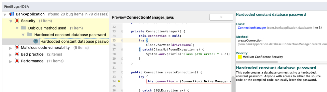
Figure 1: Static analysis tools, such as FindBugs [11], identify statements violating rules, and may also offer text explaining the rationale for the rule (bottom right).
